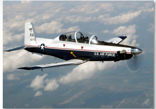
The T-6A Texan II is a single-engine, two-seat primary trainer designed to train Joint Primary Pilot Training, or JPPT, students in basic flying skills common to U.S. Air Force and Navy pilots. The trainer is phasing out the aging T-37 fleet throughout Air Education and Training Command. (U.S. Air Force photo by Master Sgt. David Richards)
